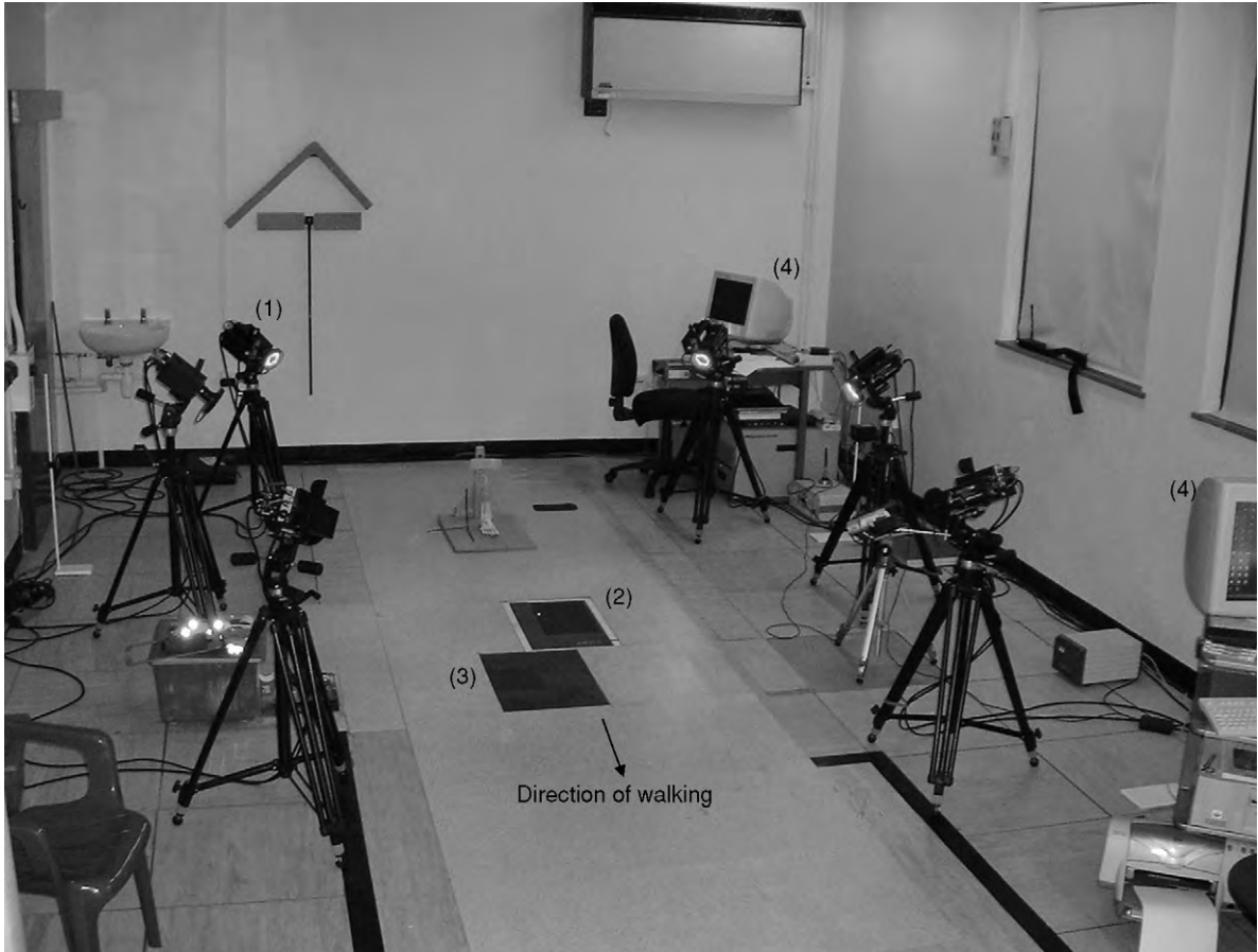
Figure 2.1 Gait Analysis Laboratory, Academic Unit of Musculoskeletal Disease, University of Leeds. Situated in the Rheumatology Outpatient Department the laboratory comprises (1) six-camera motion capture system; (2) plantar pressure distribution analysis system; (3) force plate; (4) computer workstations. Not shown are optical timing device, in-shoe pressure analysis system and instrumented walkway.
