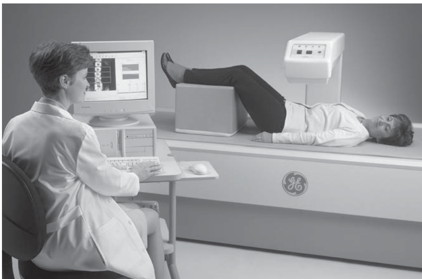
Fig. 13-6. The Lunar DPX Pro™. The newest model in the DPX series of central, pencil-beam, dual energy X-ray absorptiometers. This device is available in both a full-size and compact model. Photograph courtesy of GE Medical Systems, Madison, WI.
