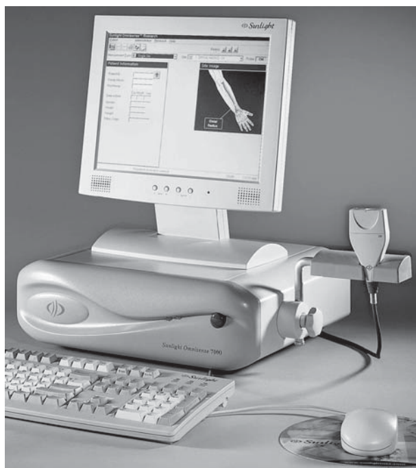
Fig. 13-28. The Sunlight Omnisense™ 7000S. A peripheral quantitative ultrasound device used to measure the radius. Photograph courtesy of Sunlight Medical Ltd., Rehovot, Israel.
