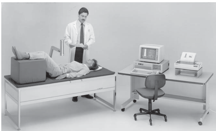
Fig. 1-8. An early Lunar DP3 dual-photon absorptiometer. This device utilized ^{153}\text{Gd} to generate photon energy. Photo courtesy of GE Medical Systems, Madison, WI.
