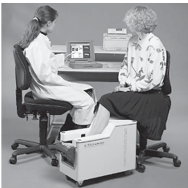
Fig. 13-26. The Osteometer DTU-one Ultrasure®. A peripheral quantitative ultrasound device used to measure the calcaneus. Shown here in use. Photograph courtesy of Osteometer MediTech, Hawthorne, CA.
