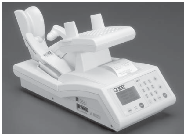
Fig. 13-30. The Quidel QUS™-2. A peripheral quantitative ultrasound device used to measure the calcaneus. Photograph courtesy of Quidel Corporation, Mountain View, CA.
